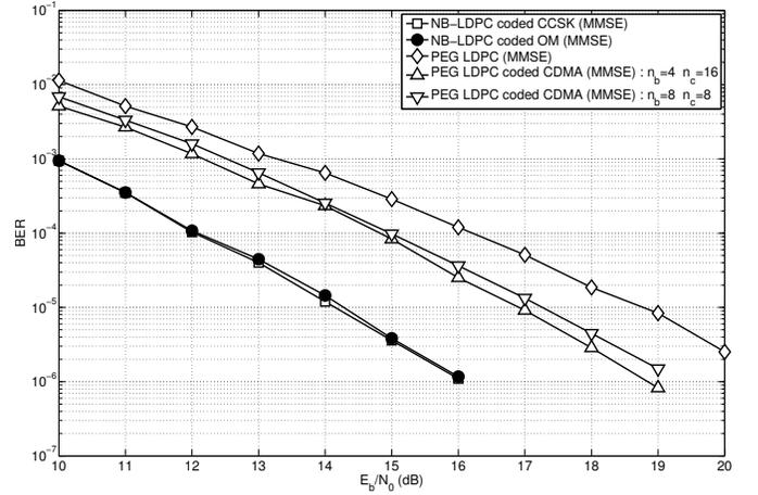
Fig. 4. BER performance of NB-LDPC coded CCSK combined with OFDM (Channel Model A)
