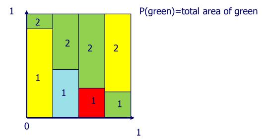
♦ X: random number between 1 to N to select color 1 (*c*<sub>1</sub>), then, read color 2 (*c*<sub>2</sub>) and the threshold *T* in a memory and compare *y* to *T* to select *c*<sub>1</sub> or *c*<sub>2</sub>.
