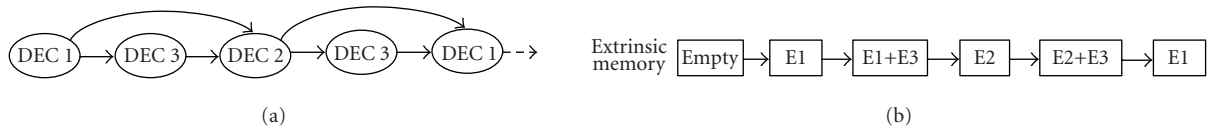
FIGURE 8: Partial serial decoding structure and extrinsic memory content (E1, E2, and E3 correspond to extrinsic information produced by dimension 1, 2, and 3, respectively).
