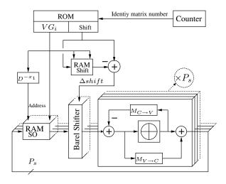
Fig. 12. Architecture of the proposed LDPC decoder
